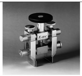
The multi-range tools have spindle actuation and a lifting mechanism with movable support jaws. Solid aluminium crossbars ensure even load distribution during the extraction operation. Their relatively large lift of approx. 15mm also permits safe extraction of arrays with bonded-on heat sinks.
